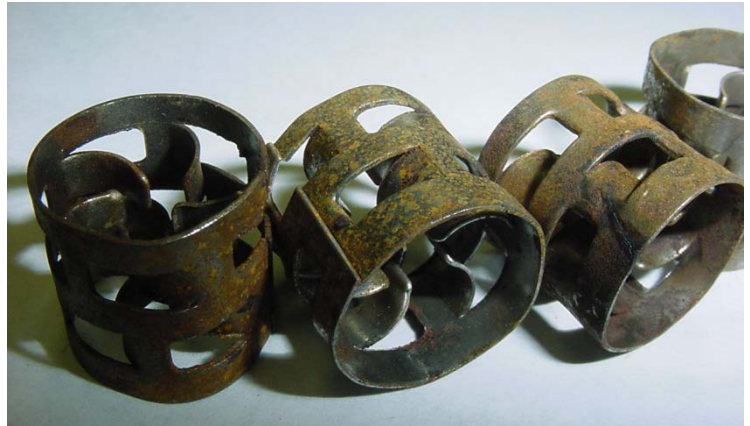
Pall Rings, L/D = 1, typical: 15 mm ≤ L ≤ 50 mm
